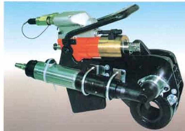
■ High speed type wrench NS system, fitted with air powered nut runner, allows high speed operation for temporary tightening and switches automatically to hydraulically bolting operation at high torque.
