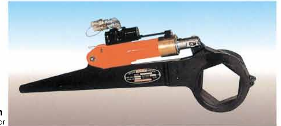
■ Hydro wrench with an extra long reaction lever The wrench body serves as the reaction point in such applications as tie rod nuts of crushers, moulding machines, etc. where distances between bolts are long.
