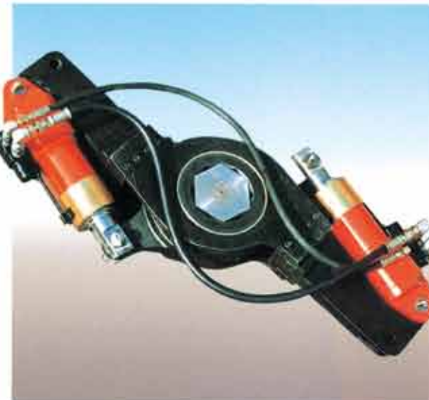
■ Twin cylinder center-hole wrench This twin system is ideal for working in tight spots and requiring higher torque force. One ratchet mechanism is driven by two cylinders to produce double torque.
