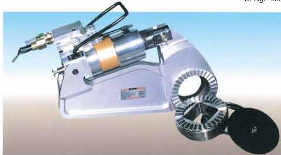
■ Titanium alloy made wrench This lightweight wrench allows easy one-hand operation to reduce fatigue and fastening time. Its weight is almost half of special steel made one.
